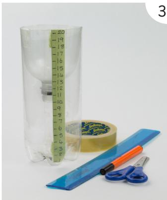
3 Make a scale in centimetres on a piece of tape, using a ruler, and fix it to the side of your bottle. You could sellotape a spare ruler on the side if you have one.
